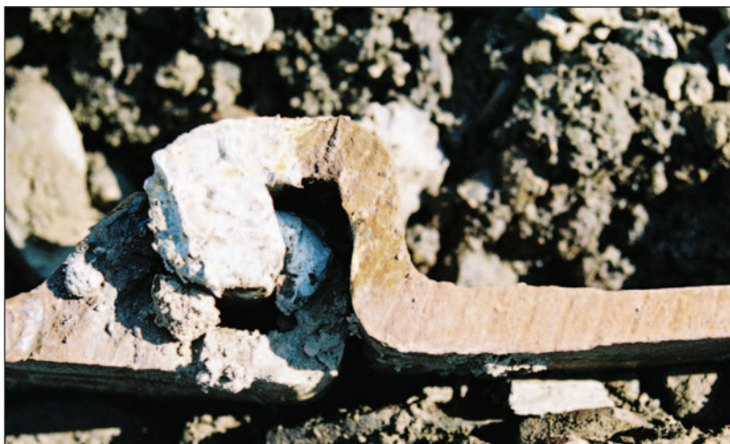
Swellseal® WA after driving sheet piles
