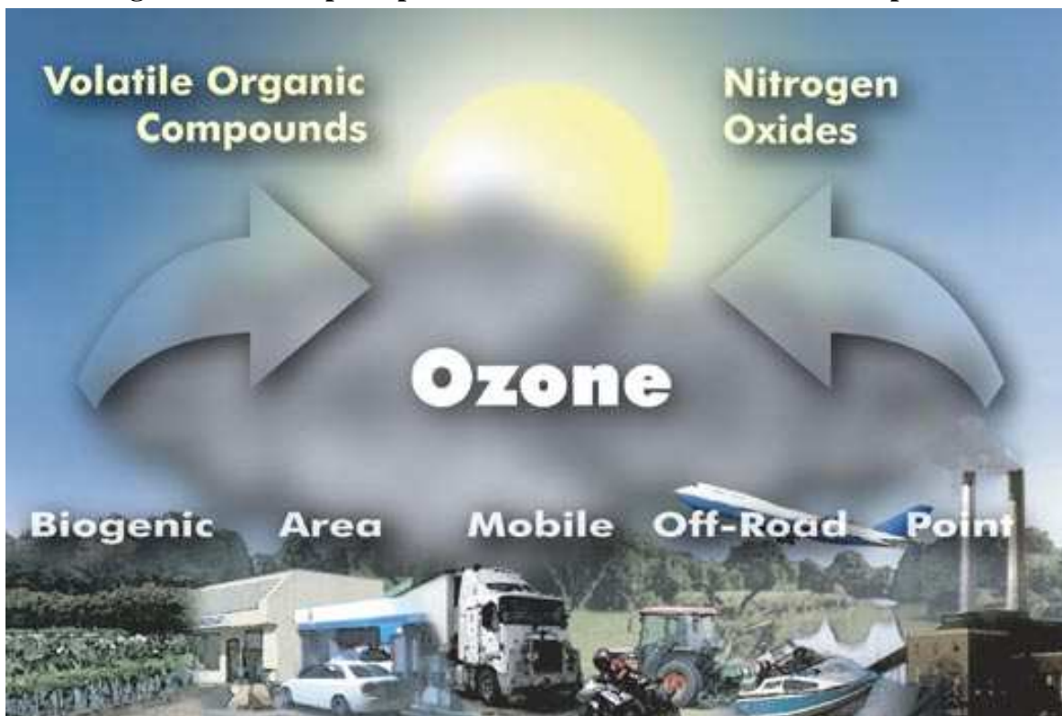
Figure 1-1. Conceptual picture of ozone formation in the atmosphere
