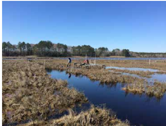
Surface elevation tables established at the Jug Bay freshwater tidal marsh to measure sediment elevation. Photo by Jenn Raulin.
