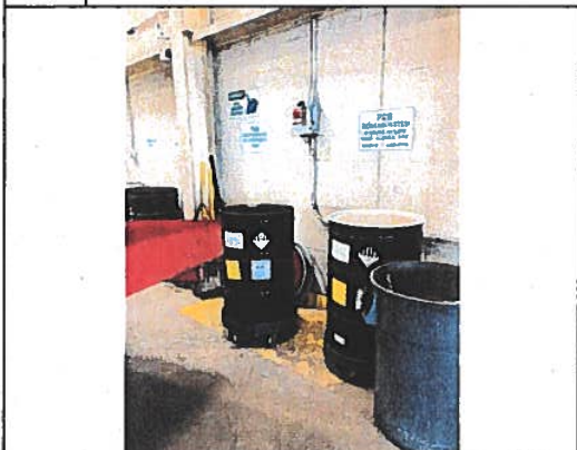
Photo #9: Storage area for used spill materials and PPE contaminated with PCBs.
