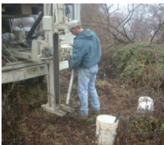
Direct push technology at work to collect a groundwater sample at the Sauer Dump site.
