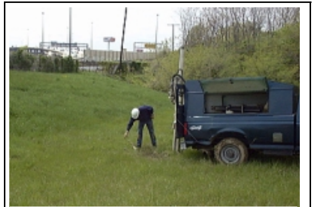
Direct-push groundwater sampling at Pemco, Inc., located in Baltimore City.
