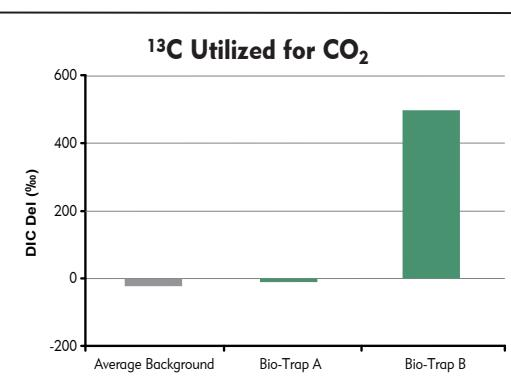
Although  $^{13}\text{C}$  incorporation into biomass demonstrated that benzene biodegradation was occurring at both locations, contaminant incorporation into biomass was substantially greater in Bio-Trap B which was consistent with a greater decrease in benzene concentration.
