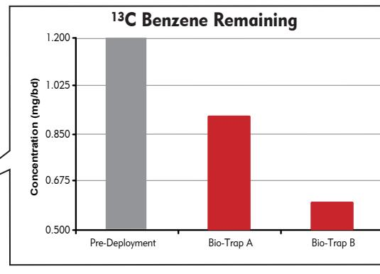
Comparison of Pre- and Post- Deployment  $^{13}\text{C}$  benzene concentrations are used to document loss of the contaminant.
