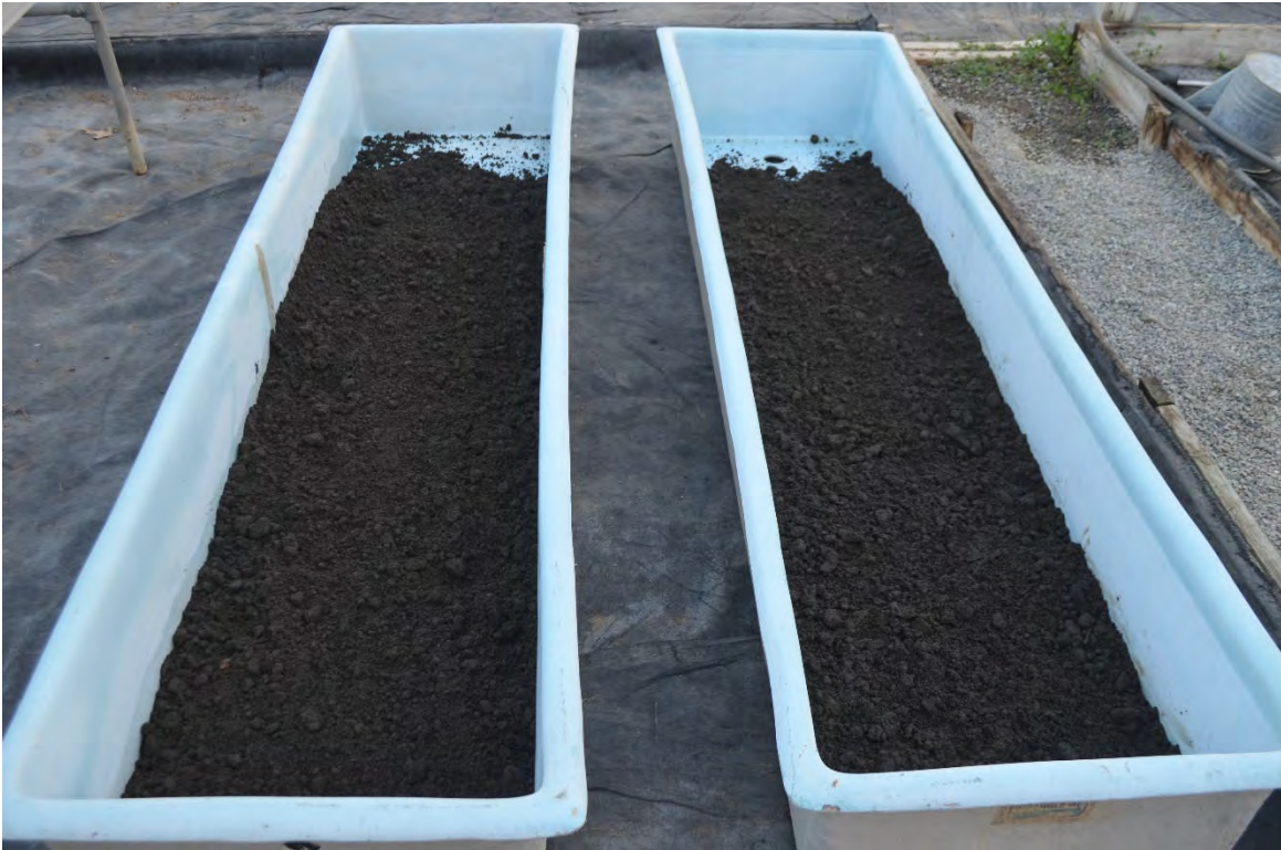
Photo 1. Conowingo reservoir sediment spread in trays to dry in preparation for creating mixes.
