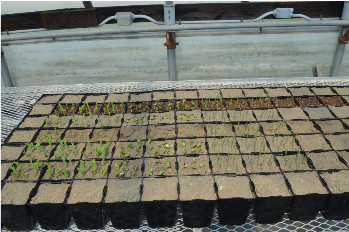
Photo 12. Full trial matrix on April 19, eight days after planting. From front to back, treatments are Leafgro mix, mushroom compost mix, poultry litter mix, unamended reservoir sediment, and peat-based commercial potting mix.
