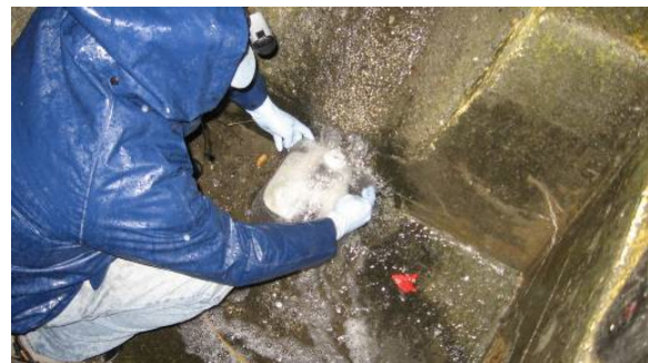
Figure 9. Collecting a sheet flow stormwater sample.
