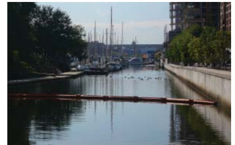
Figure 1-4. Trash Collecting Debris Boom
