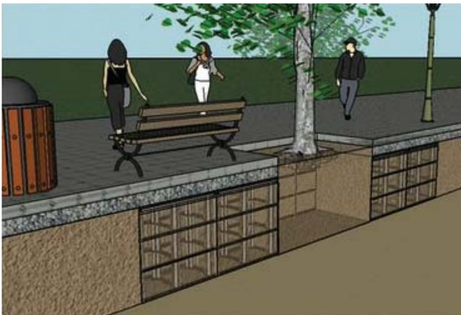
Figure 3-4. The Silva Cell system is a plastic grid which structurally supports pavement with healthy soil underneath for tree roots and water absorption. Credit: Deep Root
