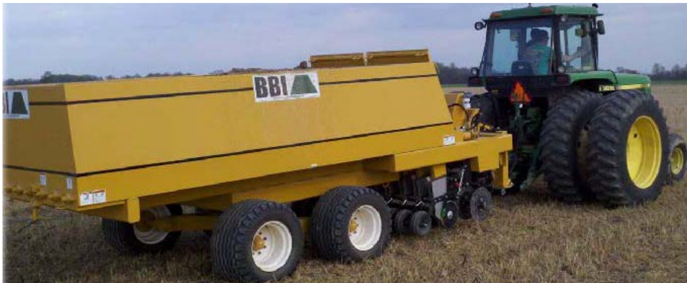
Figure 18. An innovative approach to manure nutrient management promoted by the Sassafra River Association is the “subsoiler” equipment pictured here. It is designed to carefully meter out manure being injected into the soil to match cropping needs and reduce potential for water quality impacts. The pilot project is reported for 2012 in Table 15 under Goal #20. (photo by the Sassafra River Association.)
