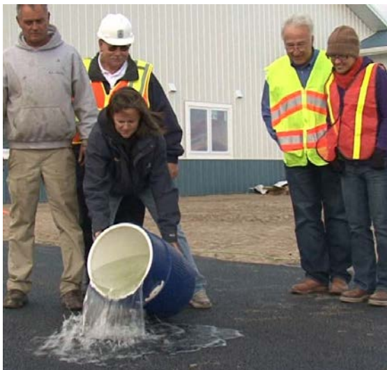
Figure 21. On a chilly day in late 2014, a local paving contractor pours water on the porous asphalt parking lot that her company recently completed for Caroline County’s new emergency services facility. This project was funded by the FFY2014 319(h) Grant to help implement the County’s Upper Choptank River watershed plan. The demonstration of water infiltration thru the parking lot surface attracted several representatives of Caroline County (standing on left) and the National Asphalt Pavement Association (standing on right). (Photo courtesy of Caroline County Planning & Codes Administration)
