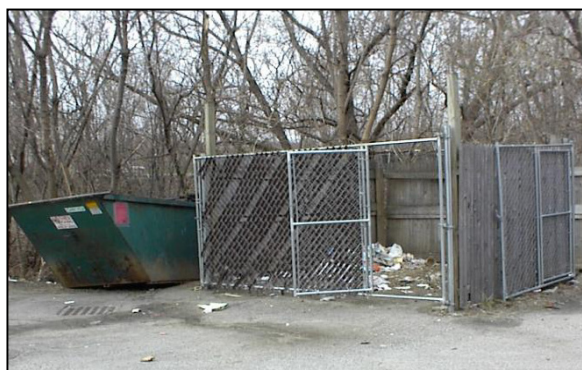
Figure 1: Dumpster Site with Typical Signs of Poor Management (trash accumulation, dumpster without lid, dumpster near storm drain)
