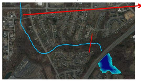
How can we determine depth of flow here with single cross section that is far upstream?
