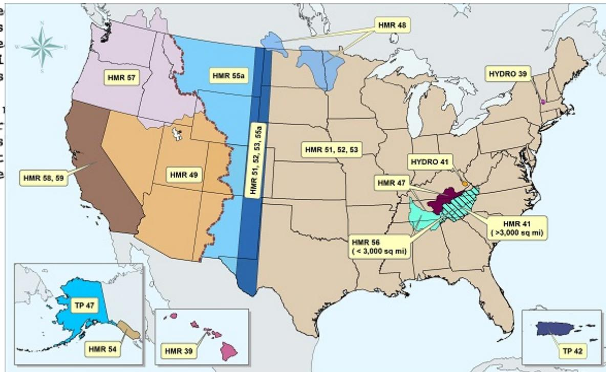
Probable Maximum Precipitation (PMP). Theoretically the greatest depth of precipitation for a given duration that is physically possible over a given size storm area at a particular geographic location at a certain time of the year.
