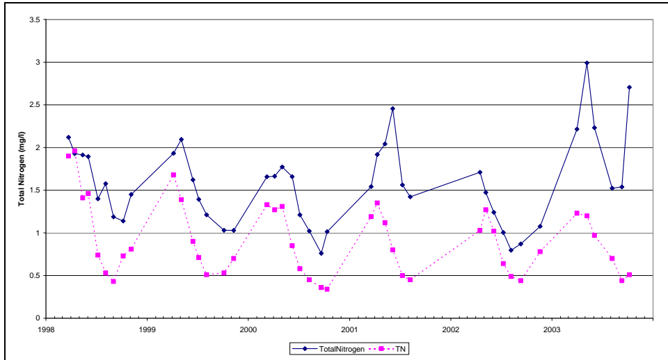
Figure C67. Observed and Simulated Average Surface Total Nitrogen Concentrations, RG1, Calibration Scenario, Rocky Gorge Reservoir
