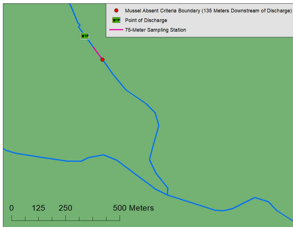
Figure 4: Sampling requirement when the distance between the point-of-discharge and the mussels absent criteria boundary is less than 150 meters
