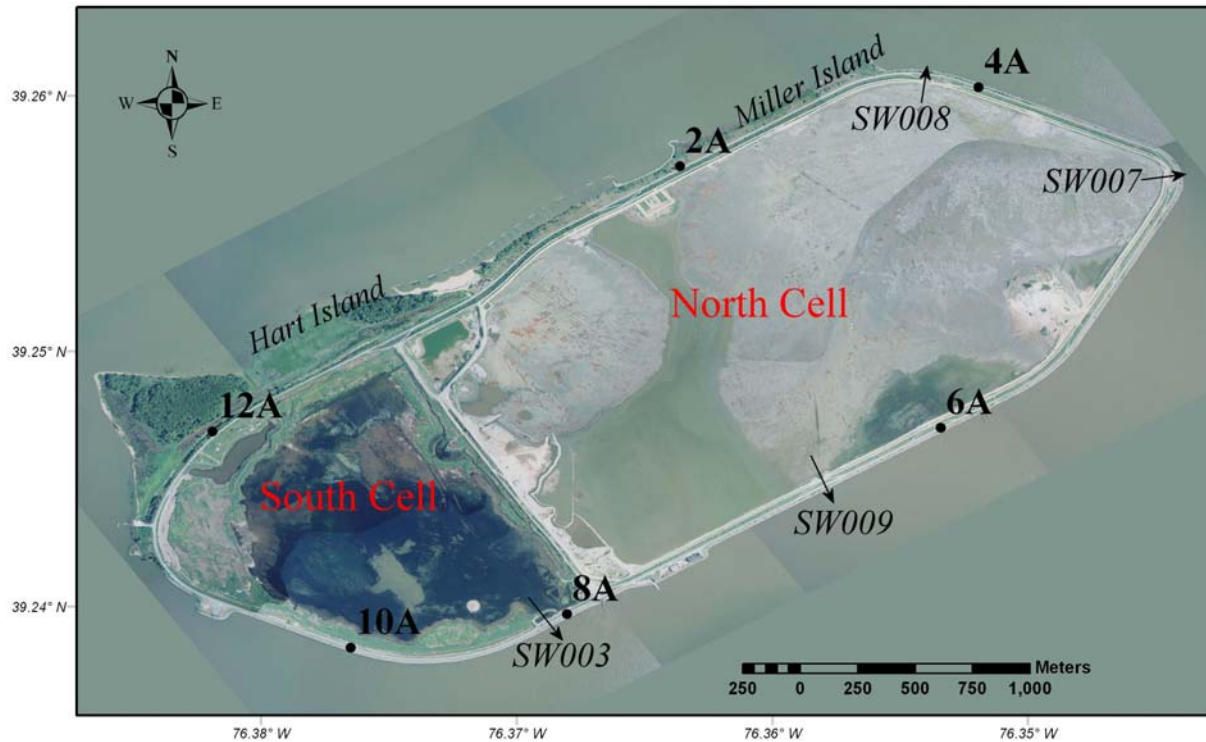
Figure 1-16. Aerial photograph of the HMI DMCF, taken on Sept. 15, 2009, showing the locations of the groundwater monitoring wells (black dots) and the spillways (SW; black arrows)..
