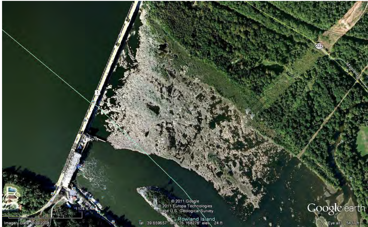
FIGURE 4.4-1: AERIAL PHOTO SHOWING ISOLATED/PERCHED POOLS IN THE CONOWINGO SPILLWAY DURING A MINIMUM FLOW RELEASE. CONOWINGO DAM OUTFLOW IN FIGURE IS APPROXIMATELY 3,800 CFS.
