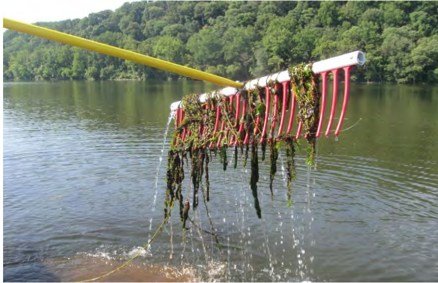
FIGURE 3.1-1. WEED RAKE USED TO CHARACTERIZE THE SAV COMMUNITY IN THE PROJECT STUDY AREA.
