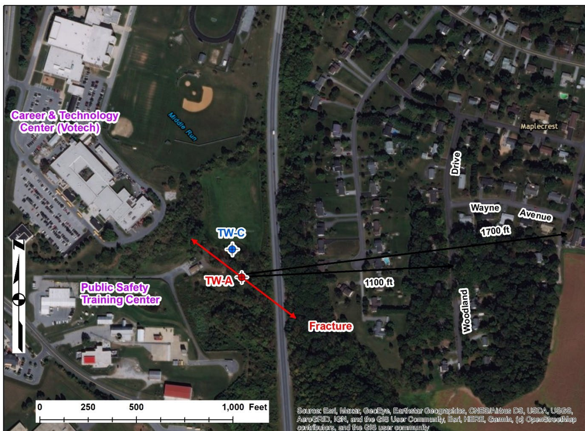
Figure 20. Imagery map for Votech well (TW-A) aquifer tests, the Maplecrest Subdivision, Career & Technology Center (Votech) and the Public Safety Training Center. The simulated fracture was derived from the Time-Distance-Drawdown calculations in the present study.
