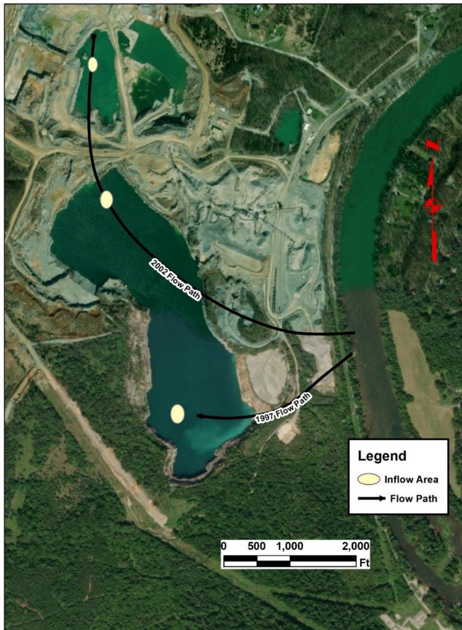
Figure 1. Aerial map of the Millville Quarry with the 1997 and 2002 flow paths from the Shenandoah River to the inflow (discharge) areas within the quarry.
