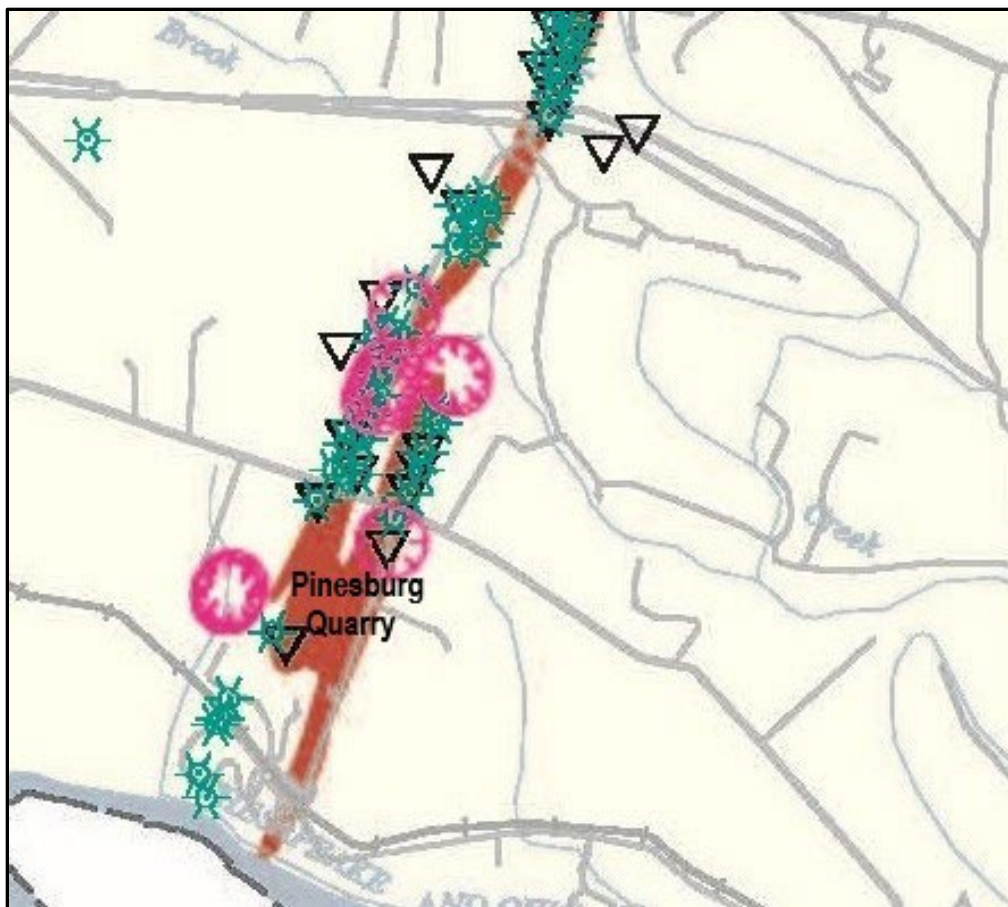
Figure 32. Location map showing karst features near the Pinesburg Quarry, modified from Duigon (2001). Pink features are collapse sinkholes.
